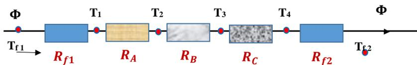
$$R_{f1} = \frac{1}{h_1 S} ; R_{f2} = \frac{1}{h_2 S}$$
