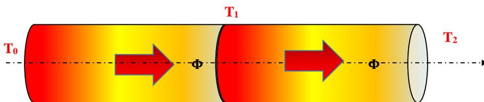
$$T_0 - T_1 = R_{th1} \Phi$$
